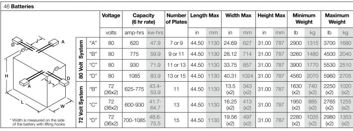
Connector Location / Length (J): A/15" (A/381mm) for all battery sizes except 80 Volt "D" Batteries require D/22" (D/559 mm). Standard Connectors: All 80 Volt Batteries = SB350 Black, All 72 Volt Batteries = SB350 Gray.
