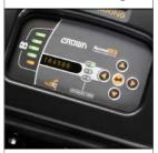
Crown's exclusive Access 1 2 3<sup>®</sup> control system enables safe, reliable, industryleading truck performance and diagnostics. It optimizes speed based on the steer angle and ensures smooth and consistent plugging, acceleration and braking.
