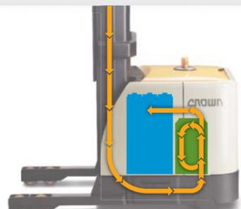
**Crown Regen Lower System** (available on SP 4000) captures lost energy and returns it to the battery. This equates to fewer battery changes, longer shifts and reduced costs.
