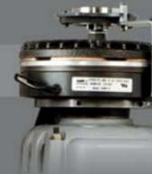
**Crown Intelligent Steering** ▲ slows the truck automatically as the steering angle increases.
