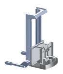
Built to outlast and outperform other brands, the SH Series features a powerful AC traction motor, heavy-duty frame and mast, steel power unit doors and a die cast aluminum handle.
