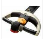
Crown's innovative X10® handle simplifies the operation of controls and reduces fatigue. The operator can quickly switch between two pre-programmed performance levels.
