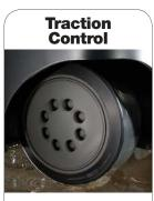
OnTrac<sup>®</sup> Anti-Slip Traction Control reduces tire spineven on wet, slick floors—improving control and extending tire life.
