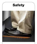
Entry Bar Safety Switch helps keep feet inside the compartment by disabling travel when depressed. In addition, the Dual Pedal Floorboard requires both feet properly positioned for travel.
