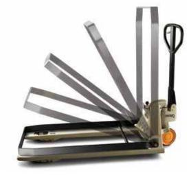
**Skid Adapter** increases lowered height to 5.5 inches to permit skid handling. Raised height increases to 10.5 inches. Adapter latches in vertical position for pallet-handling tasks.
