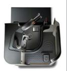
The PR 4500's compartment features five points of contact, separate brake and travel sensor pedals, and an entry-bar safety switch to enhance operator security and confidence.
