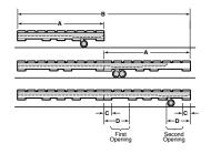
wheel, the "C" dimension should be 6" (150 mm) maximum and the "D" dimension should be 14" (355 mm) minimum. On models with tandem load wheels, the "C" dimension should be 6" (150 mm) maximum and the "D" dimension should be 17" (430 mm) minimum. Customers that need tandem load wheel trucks, but use pallets with smaller openings, may be accommodated if the maximum lift height of the truck is reduced. Contact your local Crown dealer for details.
