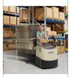
Onboard sensors monitor steer wheel angle, fork height and load weight and adjust speed and acceleration to provide safe operation and precise control.
