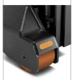
Large load wheels provide long life and are designed for easy access and replacement.
