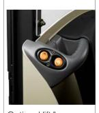
Optional lift/lower buttons mounted in the backrest offer an extra vantage point on or off of the truck for load positioning.
