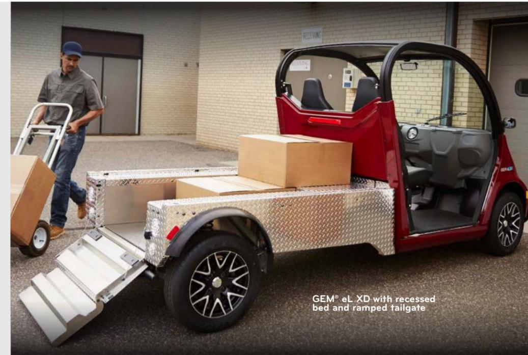
GEM® eL XD with recessed bed and ramped tailgate
