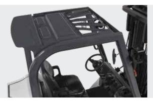
Overhead Guard Rain Cover Protects operator from rain & debris.
