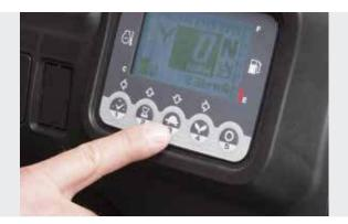
**Optional High/Low Speed Switch** Toggle from the high-speed pre-set in wide-open areas — then select the slow speed for tight environments.
