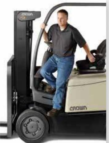
**Ease of entry/exit** saves time and improves operator productivity. The truck features convenient handholds, extra headroom, a contoured seat deck and low step height.
