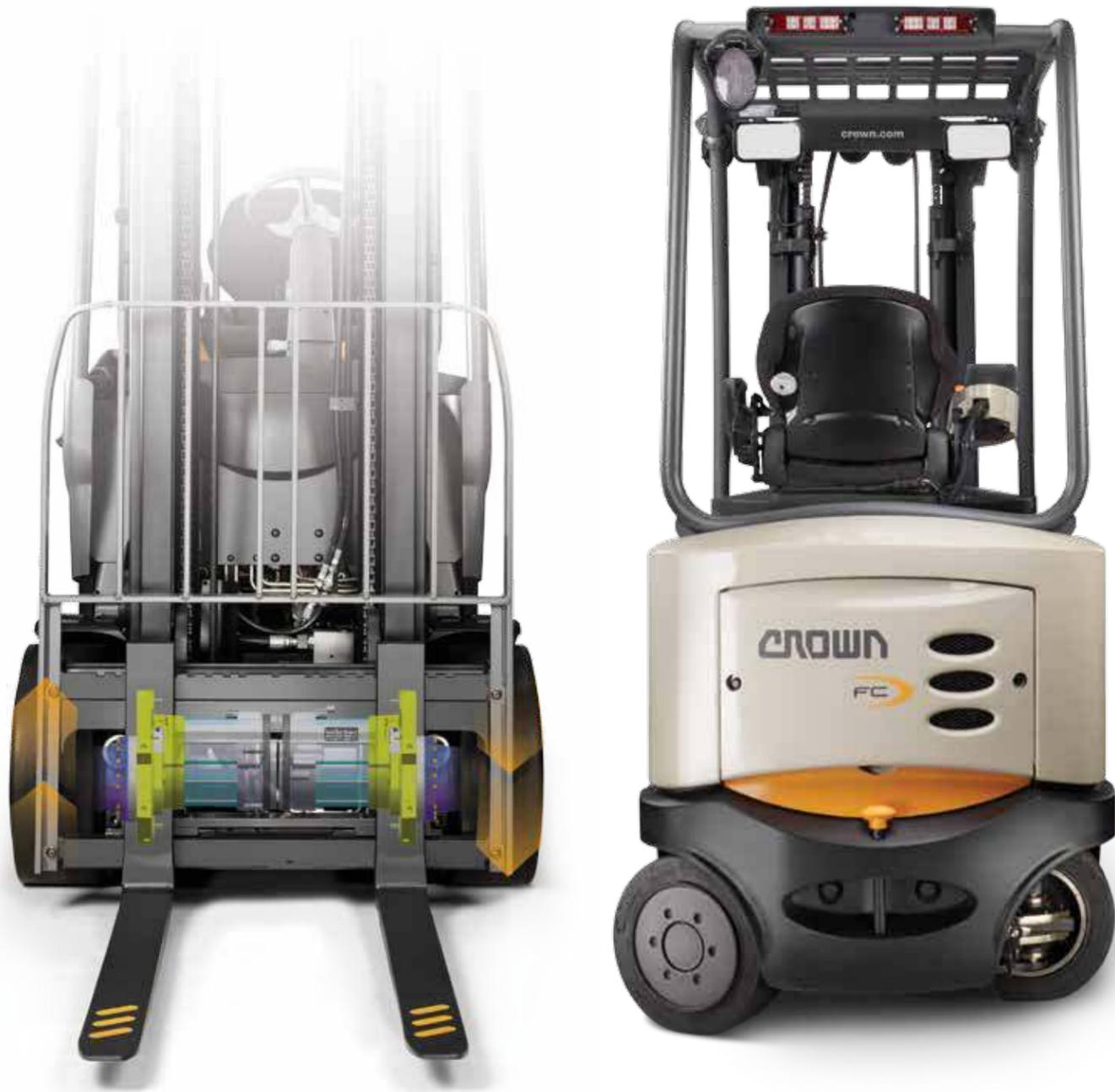
**Precise control** lets you take advantage of tighter right angle stacks. Larger, less maneuverable lift trucks require wider aisles, but drive motors turning in opposite directions allow the FC 5200 Series to spin 360 degrees in an aisle without disturbing surrounding pallets.
