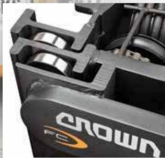
**Masts stand firm** with Crown's rigid I-beam construction, which resists longitudinal, lateral and torsional bending and twisting.
