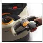
Crown's innovative X10® handle simplifies operation and reduces fatigue. The brake override feature optimizes control when maneuvering in tight areas.
