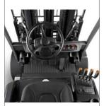
A suspension seat, tilt steering and thoughtful control placement reduce fatigue. Optional cabins with power tilting facilitate ease of service and include numerous standard features along with various options for A/C and heat, rear view camera and panoramic mirrors.
