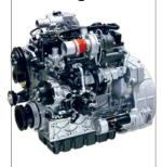
A 3.4 L Doosan diesel engine with gear-driven valve train produces 108 HP providing increased reliability and low maintenance. Compliant with Tier 4 Final exhaust emissions without the use of a Diesel Particulate Filter. Offers three performance modes: STD, ECO and Drive.
