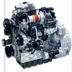
A turbocharged, intercooled 3.4 L Doosan diesel engine with gear-driven valve train produces 74 HP providing high torque at low rpm, lower fuel consumption and increased reliability. Compliant with Tier 4 Final exhaust emissions without the use of a Diesel Particulate Filter. No Diesel Exhaust Fluid (DEF) required. Two performance modes.
