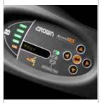
Provides onboard monitor and control of forklift systems including adjustable speed limits, operator pin codes and onboard diagnostics.
